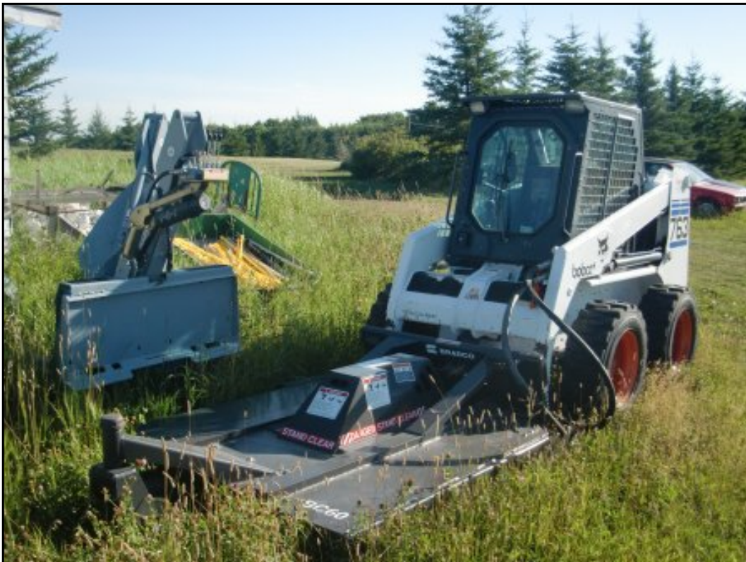
Bobcat with hydraulic lines.
