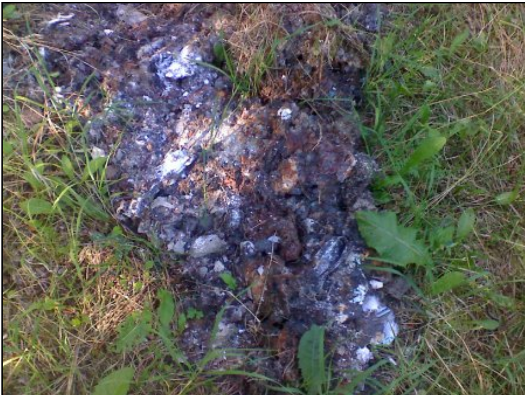
Debris pile from historical burn pit consisting of glass, metal, cinders, and unidentifiable debris.
